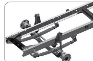
Front Parabolic Suspension and Rear Semi-elliptical Suspension
